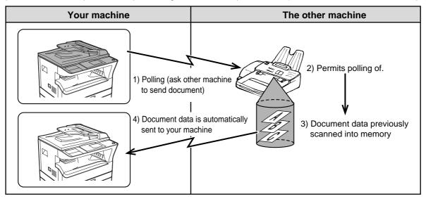
Group keys and the broadcast transmission function (page 31) can be used to successively poll multiple fax machines in a single operation (this is called "serial polling"). Up to 200 machines can be polled. In this case, the sequence of operations in the above diagram is successively repeated for each sending machine selected.
